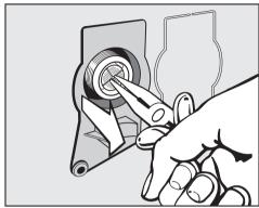
■ Use flat pliers to pull the filter out by the fin, and clean it. Reverse the instructions to re-insert and secure the parts.
